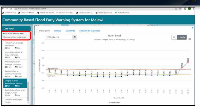
Alarm and siren is activated when the telemetric water level reaches the Warning Level
